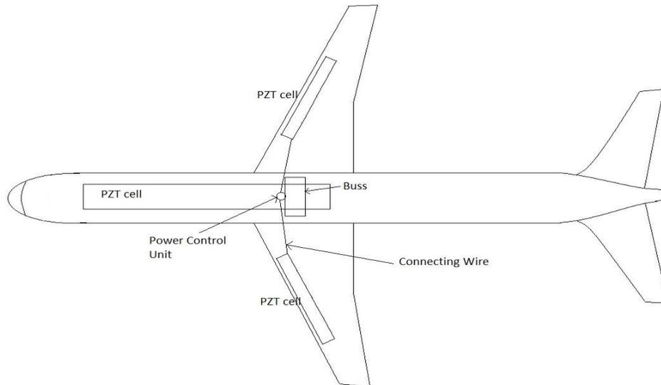
To make the system more economical the use of connecting wire is very remarkable. Using economical wires at the same time not compromising the safety factors is the effective process which is likely to be achieved. Another point is that the installation of the Power Control Unit and Bus should be in a position that the distances from all the unit cell are minimum. This will reduce the use of wire and eventually the cost.
