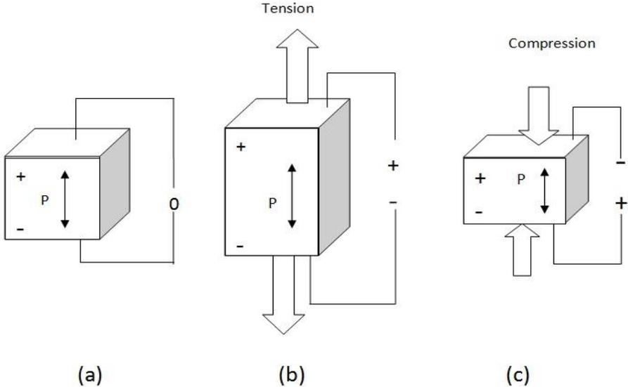
Figure 2: Electric Dipoles in Piezoelectric Material Before, During and After Poling
