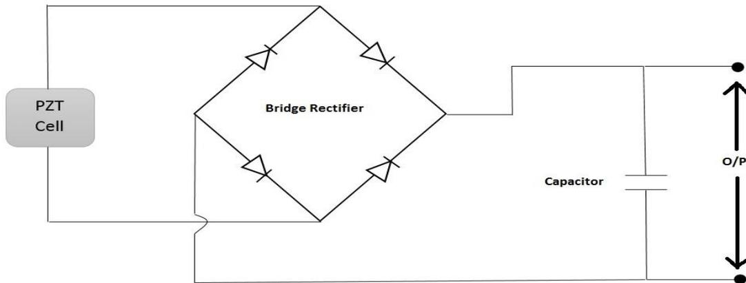
A capacitor with a high Farad value is connected in parallel to the output of the rectifier in order to accumulate charges in the plate of the capacitor. This helps to provide a regular and steady current flow which is desired to be achieved. All the other unit cells are treated as the same.
