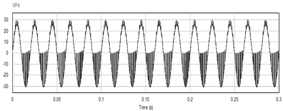
Figure 7: Output Voltage of the Pure Sine Wave Inverter before Using Filter
