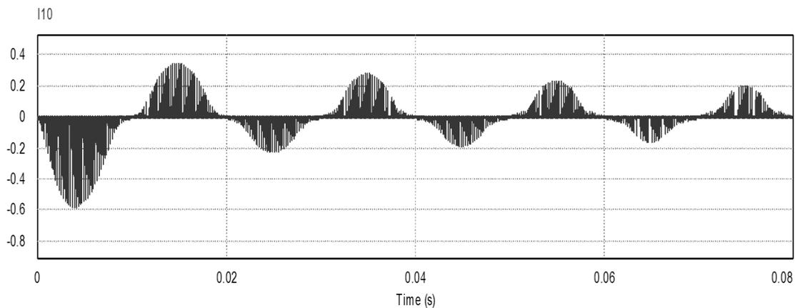
Figure 5: Input Current before Filtering
