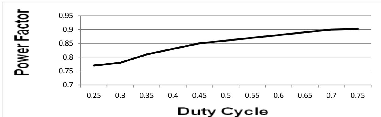
**Figure 11: Power Factor Vs Duty Cycle for Pure Sine Wave Inverter's Gate Pulse When The Rectifier's Duty Cycle is Fixed At 0.25.**
