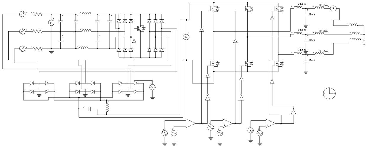
**Figure 3: Schematic Diagram of Proposed Combined Circuit of Three Phase Buck Rectifier and a Pure Sine Wave Inverter**
