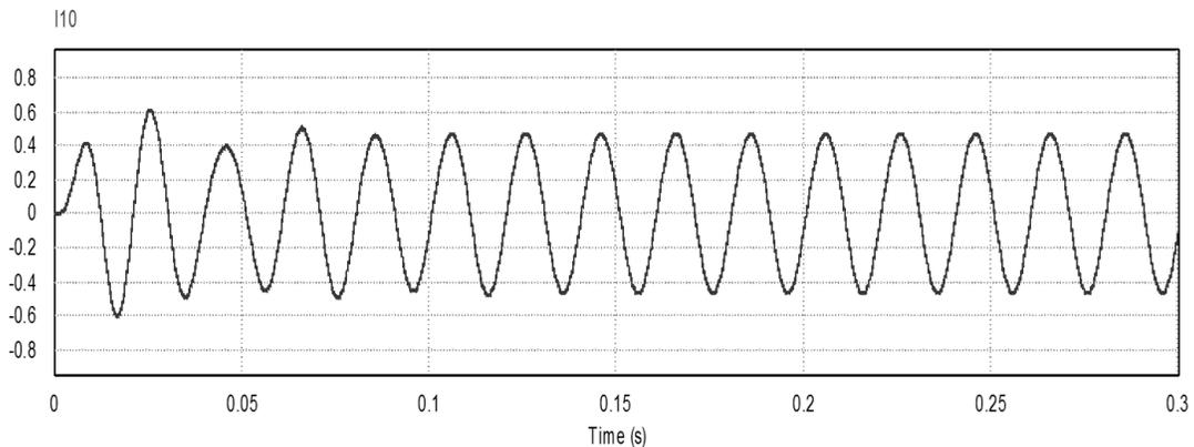
**Figure 10: Output Current of Highly Efficient Pure Sine Wave Inverter after Filtering**
