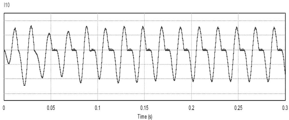
**Figure 9: Output Current of Pure Sine Wave Inverter before Using Filter**
