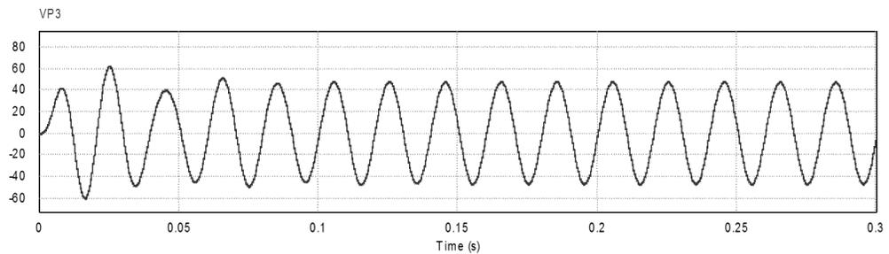
Figure 8: Output Voltage of Highly Efficient Pure Sine Wave Inverter after Filtering
