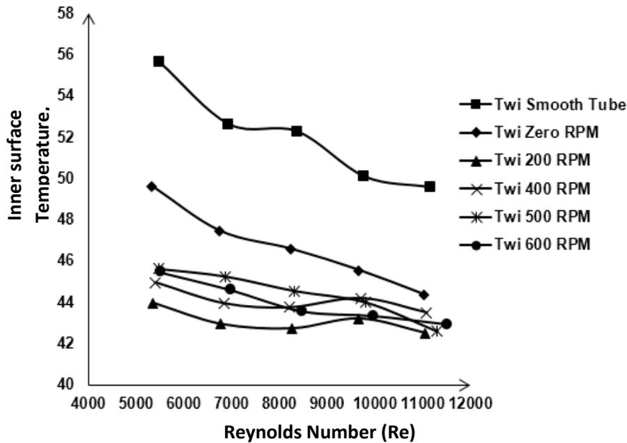
**Figure 4: Variation of Inner Surface Temperature with Reynolds Number for Different Flow Rate and Rotation of Twisted Tape**
