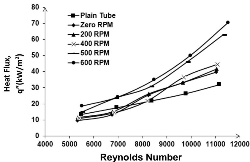
Figure 3: Variation of Heat Flux with Reynolds Number for Different Flow Rate and Rotation of Twisted Tape.
