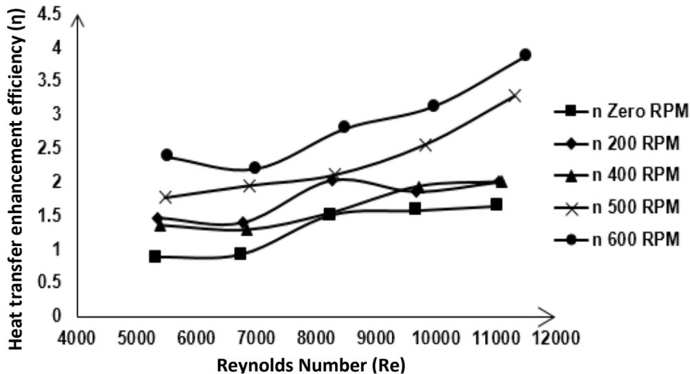
**Figure 5: Variation of Heat Transfer Enhancement Efficiency with Reynolds Number for Different Flow Rate and Rotation of Twisted Tape.**
