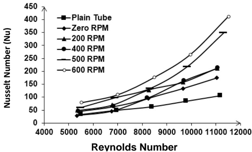
Figure 2: Variation of Nusselt Number with Reynolds Number for Different Flow Rate and Rotation of Twisted Tape.
