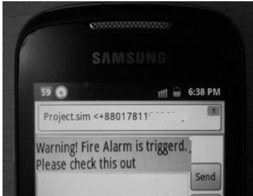
Figure 7: Snapshot of SMS When Fire Sensor is Triggered
