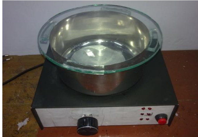
Figure 1: Complete Setup of a Simple Spin Coater
