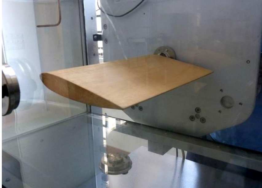
Figure 6: Photograph of Cambered Aerofoil (NACA 4415)
