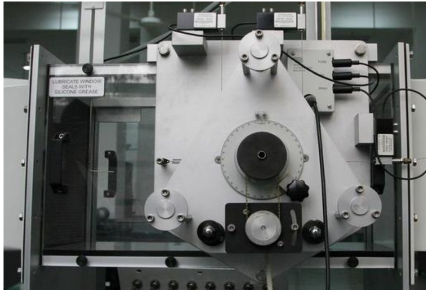
Figure 10: Working Section with Three Component Balance of Wind Tunnel.
